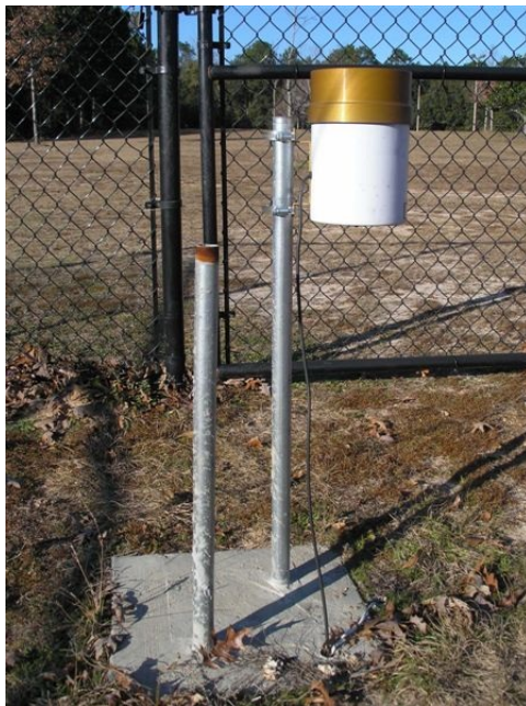
Figure 3. University of South Alabama Mesonet tipping bucket rain gauges: a) Hydrological Services TB3 and b) Texas Electronics TE525. Photographs taken at USA Campus site by S. Kimball.
