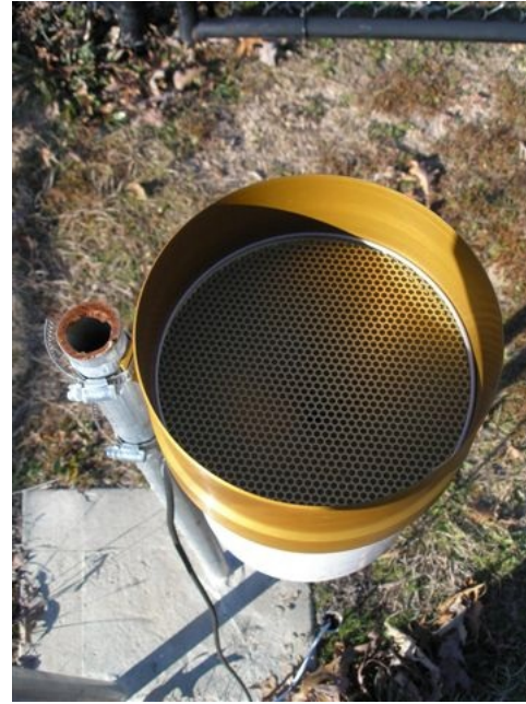
Figure 3. University of South Alabama Mesonet tipping bucket rain gauges: a) Hydrological Services TB3 and b) Texas Electronics TE525. Photographs taken at USA Campus site by S. Kimball.
