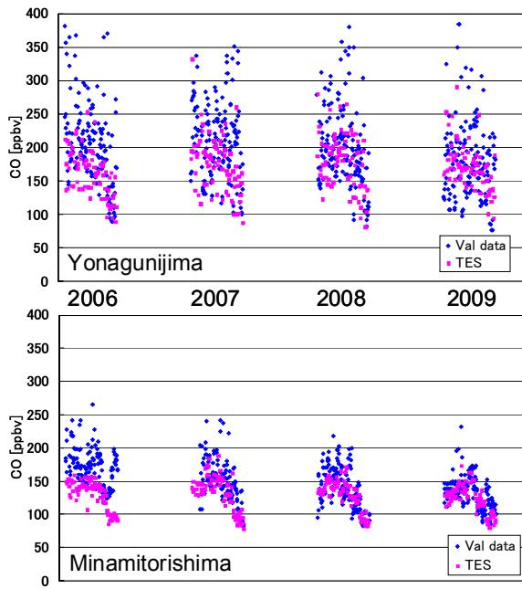
Figure 4. The comparison of TES level3 CO product and in-situ data in January-May from 2006 to 2009 at Yonagunijima (above) and Minamitorishima (below).
