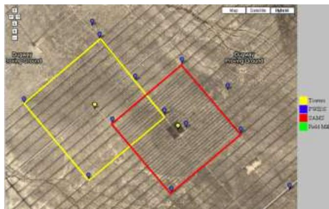
Figure 1. Map of instrumentation showing location of existing test grid (red square), proposed new test grid (yellow square), towers (yellow icons), and PWIDS (blue icons).
