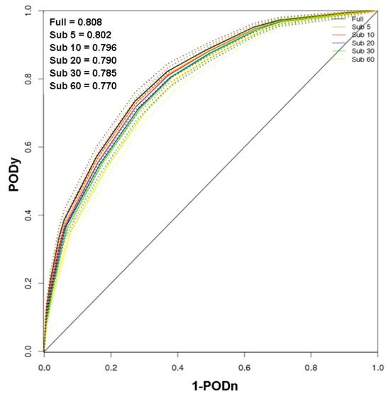
**Figure 6:** Receiver Operating Characteristic (ROC) plot for GTG2 product using EDR observations. The legend is located in the top right. Area under the curve (AUC) calculations are in the top left corner.
