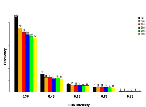
**Figure 2:** Distribution of Moderate-or-greater (MOG) EDR observations color coded by sub-sampling rate. Frequency of occurrence is normalized frequency. N samples observed are at the top of each bar graph with the legend in the top right.
