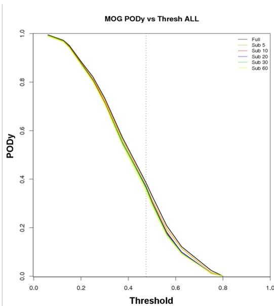
**Figure 5:** Dichotomous Probability of Yes Detection (PODy) score for GTG2 product using EDR observations. The GTG2 Moderate-or-greater threshold is indicated by the dashed vertical line. The legend is located in the top right.
