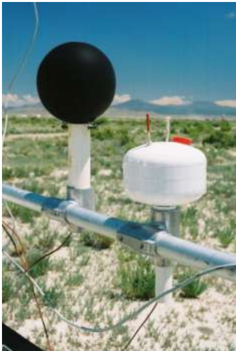
Fig 2.1 Black Globe and Natural Wet Bulb sensors used at Dugway Proving Ground
