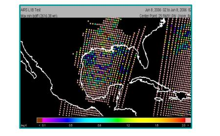
AQUA AIRS clear FOR search module -Utilizes spatial coherence test threshold for clear ocean detection As confidence in VIIRS and CrIS geolocation is gained, VIIRS data can be used to identify clear CrIS FOVs
