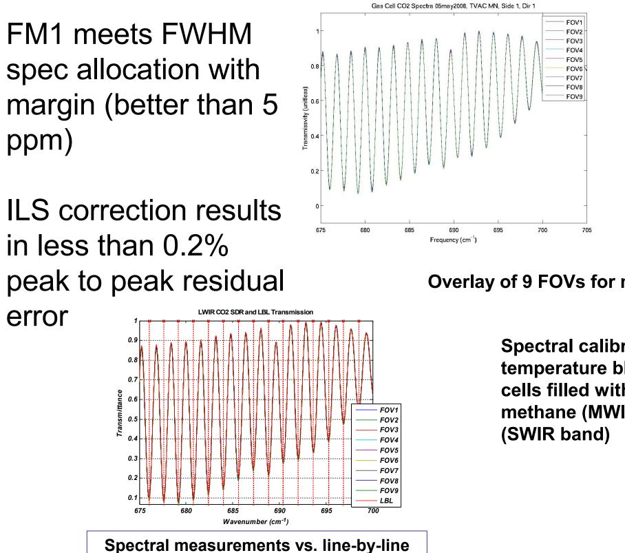
Frequency (cm<sup>-1</sup>) Expanded view at 682 cm<sup>-1</sup> **Overlay of 9 FOVs for measured CO<sub>2</sub> spectrum** Spectral calibration is determined from hot temperature blackbody measurements of gas cells filled with carbon dioxide (LWIR band),
