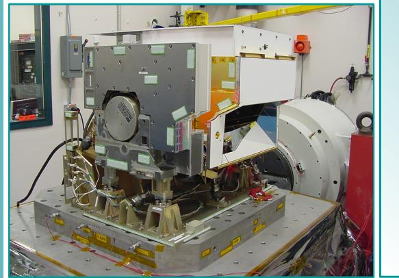
Key Technical Aspects of CrIS: Fourier Transform Spectrometer 14 km nadir FOV spatial resolution Fields of Regard with 3 x 3 FOVs Photovoltaic Detectors in 3 bands 4-Stage Passive Detector Cooler 2200 km swath width On-board internal calibration target (ICT) Supplier: ITT
