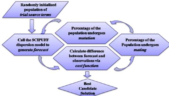
Figure 6. The Genetic Algorithm (GA) procedure.
