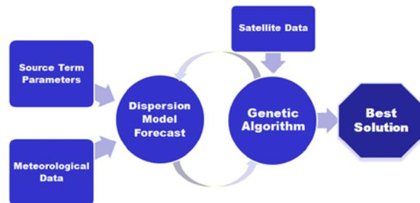
**Figure 2. Source Term Estimation Solution Process.**
