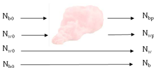
Figure 2. Geometry defining the variables for computing opacity by (1).
