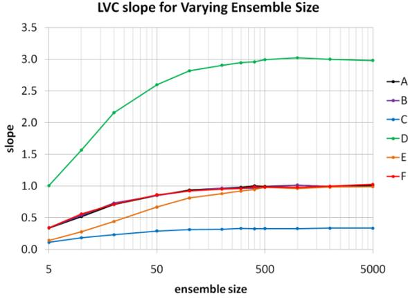
Figure 3: Calculated LVC slope for each of the experiments listed in Table 1 using variable ensemble sizes. The theoretical slope is 1 for Exps. A, B, E and F;  $\frac{1}{3}$  for Exp. C; and 3 for Exp. D. Data are plotted at ensemble sizes of 5, 10, 20, 50, 100, 200, 300, 400, 500, 1000, 2000 and 5000.
