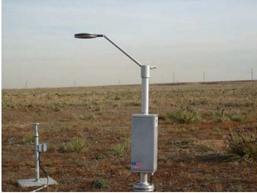
Figure 2 - Yankee Environmental Systems Inc. Hotplate precipitation gauge.
