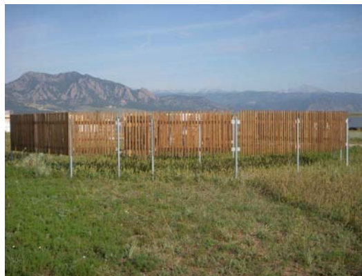
Figure 1 - GEONOR precipitation gauge in a DFIR shield.
