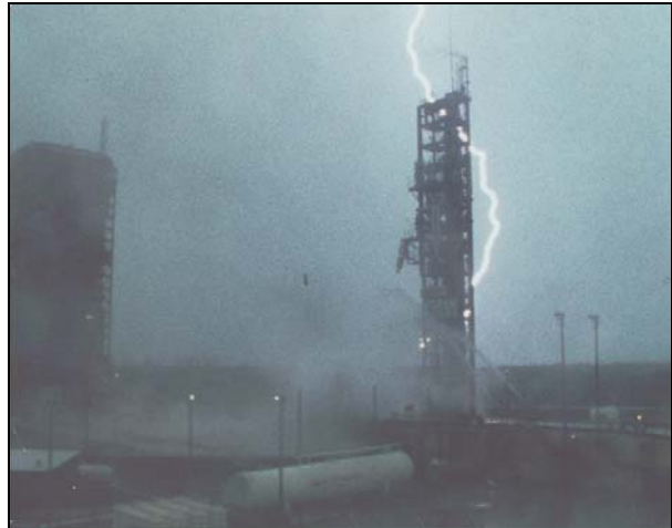
Figure 1. Triggered lightning strike to the in-flight Atlas/Centaur-67 mission on 26 Mar 87. Shown here is the triggered lightning following the exhaust plume to the ground at the launch pad. The space launch vehicle and payload were destroyed as a result of this triggered lightning.
