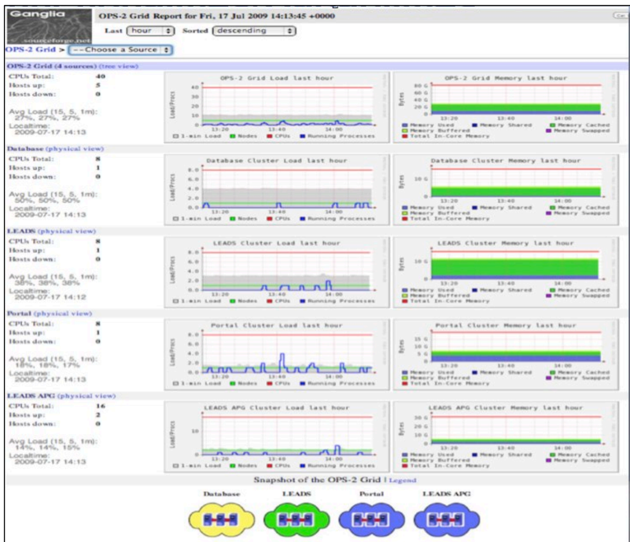
FIG. 14. Ganglia display page, depicting color-coded memory, load, and other trends of system statistics for all components of a specific hardware thread. Each hardware thread has its own Ganglia instance, but Belgocontrol system administrators can monitor all instances simultaneously.
