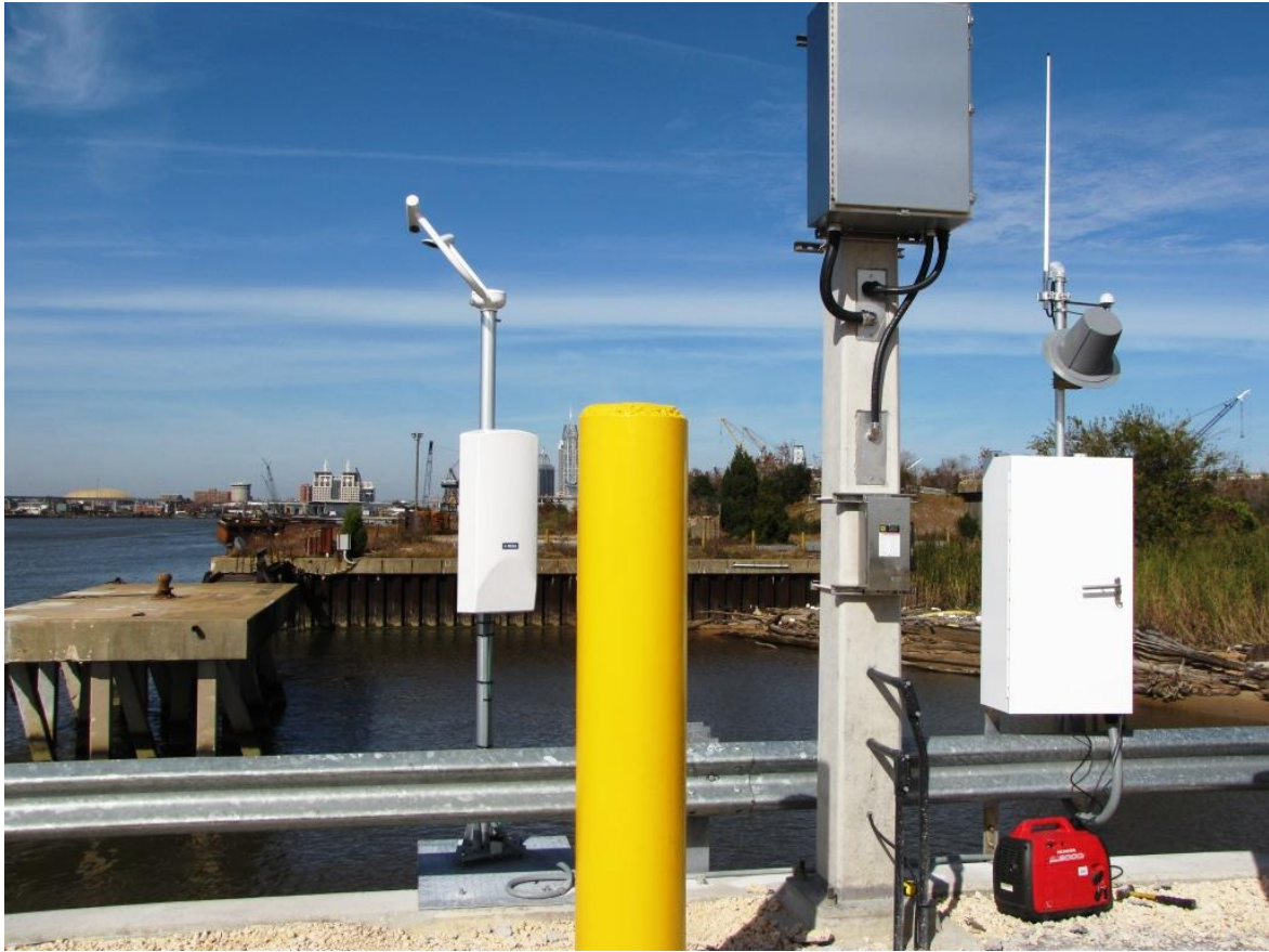
Figure 2. Vaisala FS11 visibility sensor installed at Pinto Island Terminal, Mobile AL
