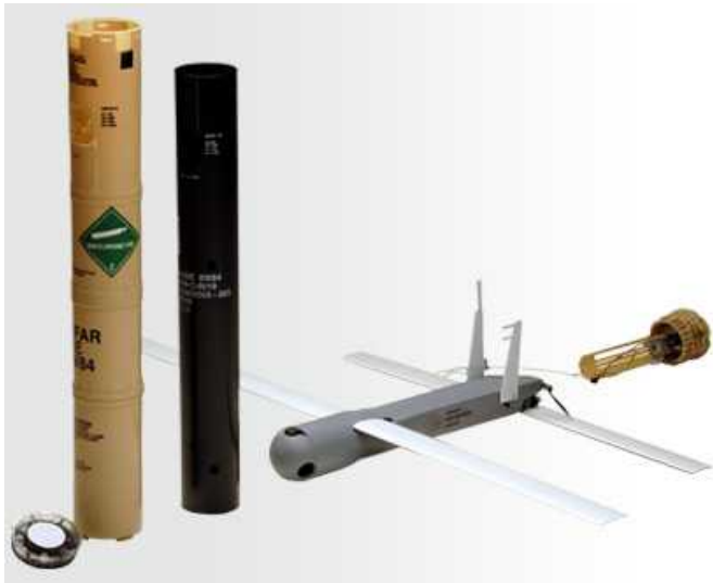
Figure 9 The Coyote unmanned aerial system that was successfully launched and controlled from a NOAA WP-3D in the summer of 2009.
