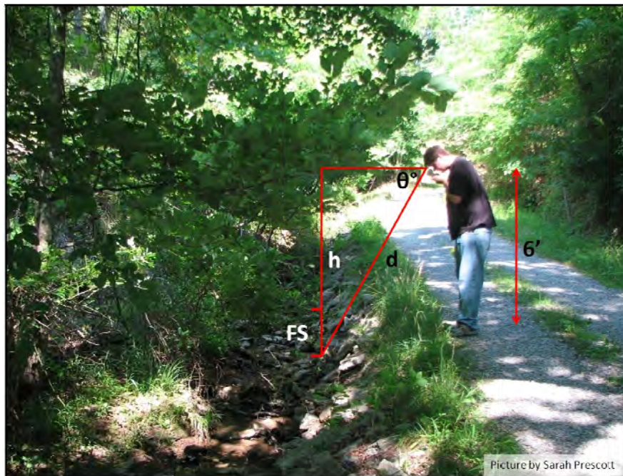
Figure 2. The author taking measurements and an overlay of how to calculate flood stage.
