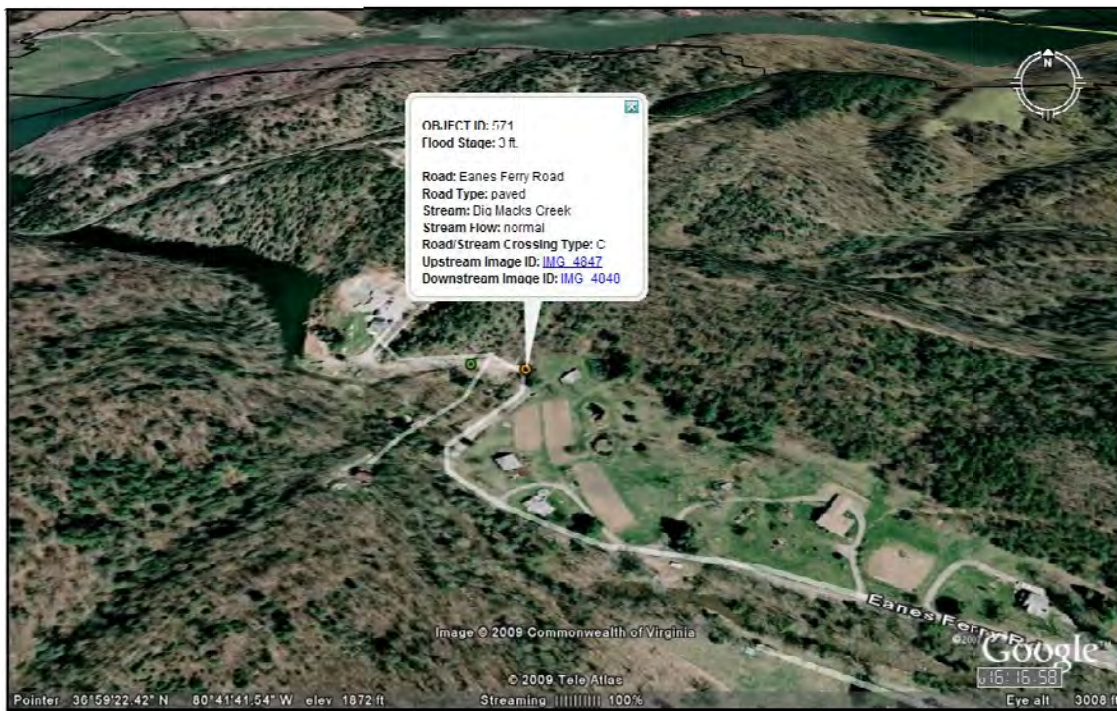
Figure 6. Google Earth overlaid with surveyed points and accessible information. Not shown in picture: Average Daily Traffic Count information which is readable in actual kml file.
