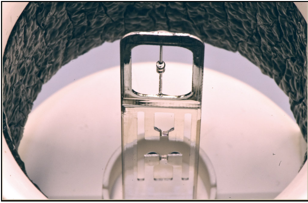
FIGURE 3. Close-up view of the pressure, temperature, and humidity sensors in the RD94 dropsonde.
