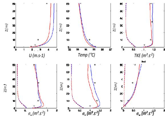
Figure 4 Comparison of Meso-NH model with (red) and without (blue) the drag force implementation over the Lannemezan 2005 experimental site. Mean vertical profiles of horizontal wind velocity (a); temperature (b); turbulence kinetic energy (c) (total : solid line, sub-grid : long dashed) ; and standard deviations of the three wind components (d,e,f) (total : solid line, sub-grid : long dashed).
