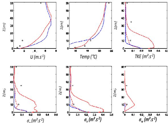
Figure 5 Comparison of Meso-NH model with (red) and without (blue) the drag force implementation over the Lannemezan 2005 experimental site. Mean vertical profiles of mean horizontal wind velocity (a); temperature (b); turbulence kinetic energy (c) (total : solid line, sub-grid : long dashed) ; and standard deviations of the three wind components (d,e,f) (total : solid line, sub-grid : long dashed).
