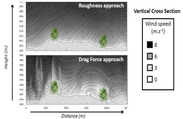
Figure 3 Vertical cross section of instantaneous wind fields simulated with roughness (a) and drag force approach (b).
