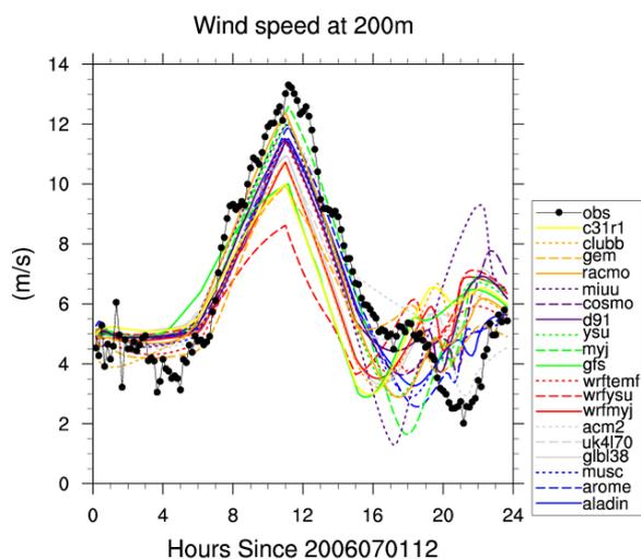
**Figure 3.** Wind speed at 200 m for the models together with observations.
