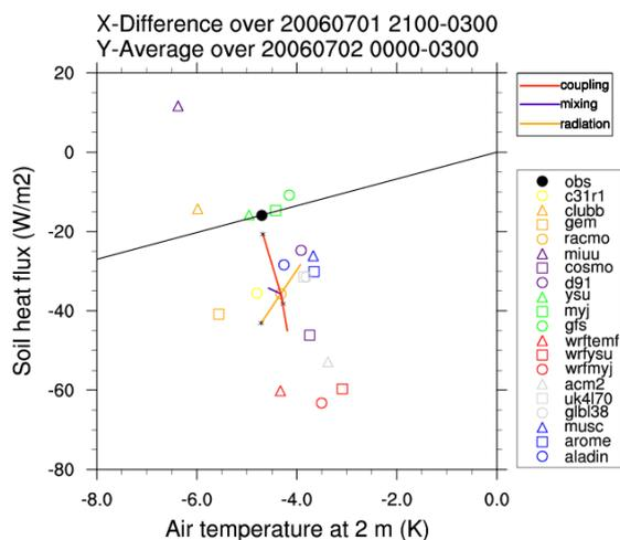
**Figure 5.** Night time soil heat flux as function of 2m air temperature change over the night. The black line represents points with the same coupling as observed. The three colored lines connect the different sensitivity runs (see main text). The crosses at the colored lines represent the points with lowest coupling, mixing and radiation respectively.
