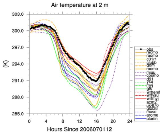
**Figure 2.** Air temperature at 2 m for the models together with observations.
