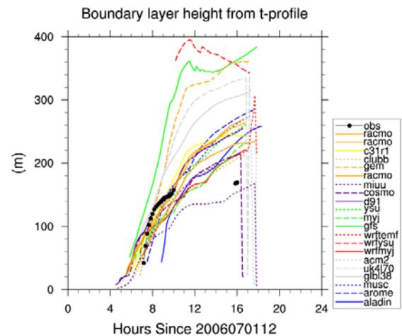
**Figure 4.** Stable boundary layer height, based on air temperature maximum, as function of time.
