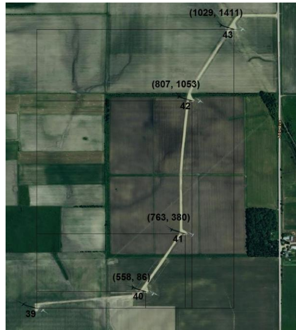
Fig. 1. Layout of the southwestern portion of the wind farm and placement of the sodars.
