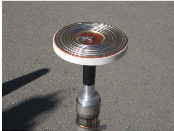
Fig 2c. Hotplate to ensure a 1 minute response for high snow rates with extreme blizzard conditions (below).
