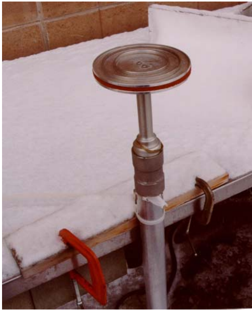
Fig 2c. Hotplate to ensure a 1 minute response for high snow rates with extreme blizzard conditions (below).
