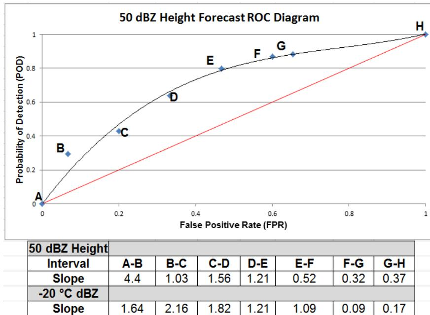
**Fig. 7 – The results of the calculation of slope intervals for each method are listed in the table. Each point on the ROC diagram is labeled A-H beginning at the origin. The calculated slopes represent the slopes of each line segment between successive points.**
