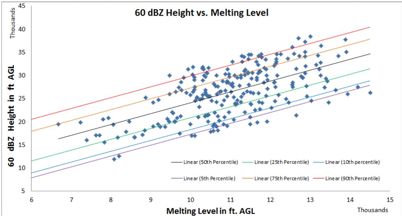
**Fig. 3 - The 60 dBZ height hail detection method with the 90<sup>th</sup>, 75<sup>th</sup>, 50<sup>th</sup>, 25<sup>th</sup>, 10<sup>th</sup>, and 5<sup>th</sup> percentile linear regression lines plotted.**
