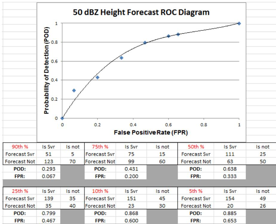
**Fig. 5 - An example of the creation of a ROC diagram using scoring from the 50 dBZ height hail detection method. Each threshold is labeled in the table in red text.**
