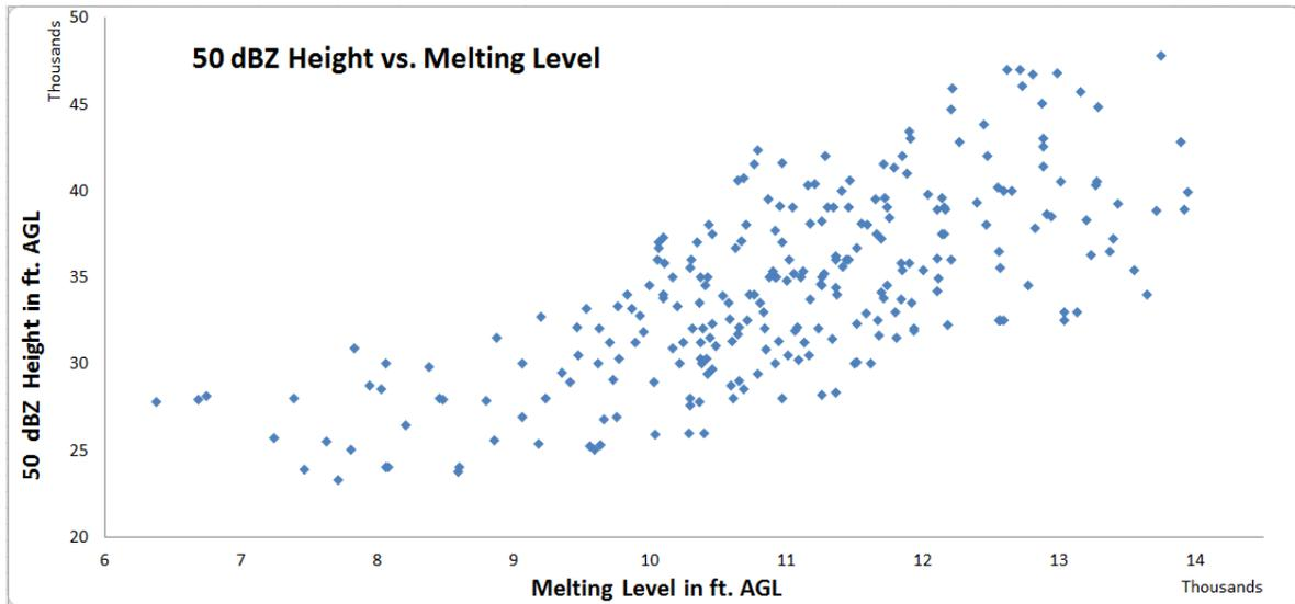
**Fig. 2 – The melting level plotted as a function of the altitude of the 50 dBZ reflectivity echo in feet AGL. The plotted data are the 260 storms that make up the training database from 2008. The majority of the data fall between the 8,000 and 13,500 ft melting levels.**
