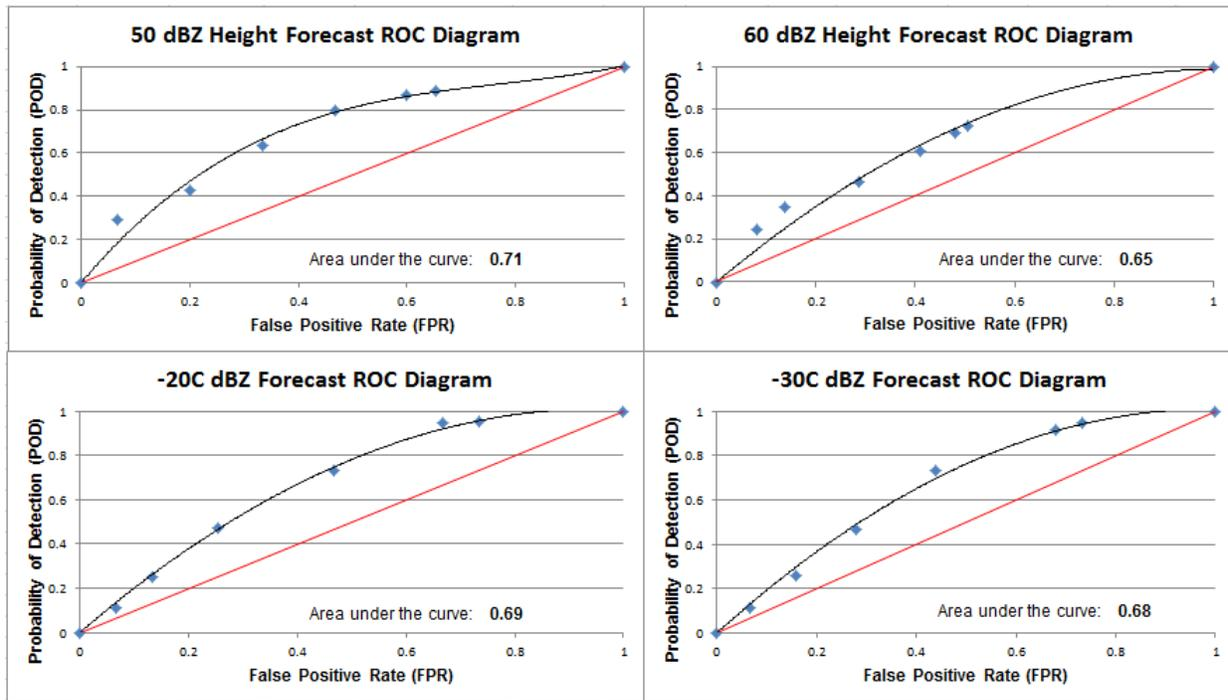
**Fig. 6 – The ROC curves for each hail detection method with the area under the curve displayed in the bottom right corner of each diagram. The red line in each diagram represents the ROC curve corresponding to a hail detection method with zero skill at discriminating severe hail producing storms.**
