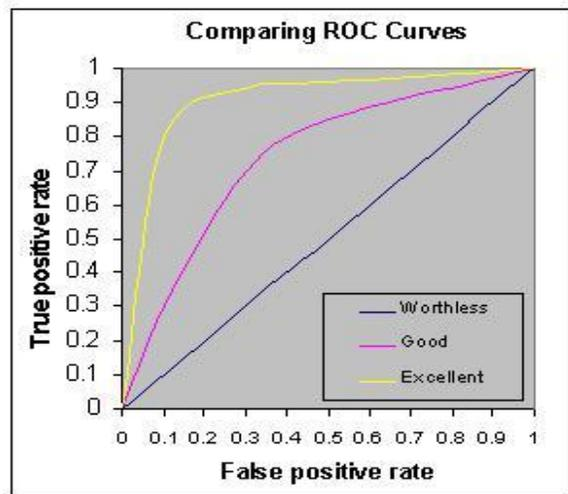
**Fig. 4 - The graph represents what ROC curves would look like for a diagnostic test whose ability to discriminate between 2 classes can be described as "worthless", "good" and "excellent". Note that a diagonal line represents a test with no skill and a curve closer to the upper left hand corner represents a nearly perfect test. (From Tape, 2001)**
