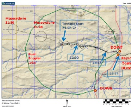
Figure 14. (above) The DOW6 and DOW7 dual-Doppler lobe during the genesis, intensification, and dissipation of the 5 June 2009 tornado. The rapid-scan DOW captured high-resolution data during tornado intensification and demise.
