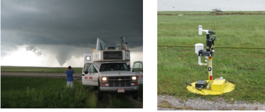
Figure 9. (above) The Rapid-Scan DOW observing a tornado on 05 June 2009 in Wyoming during VORTEX2(left). An instrumented Tornado Pod (right).
