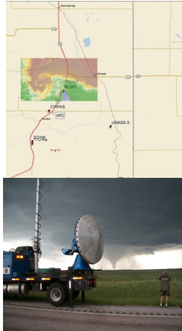
Figure 7. (right)(top) Actual deployment of several of the VORTEX2 radars near a tornado on 05 June 2009 in Wyoming. The DOW6 and DOW7 radars are collecting dual-Doppler data. The UMASS-X and NOXP radars are deployed ahead of the storm to collect storm-scale and later mesocyclone scale data as the storm moves east. The DOW5/Rapid-Scan is collecting ultra-fine-scale data at ranges as low as 400 m. The CIRPAS phased array, The SMART-Radar 2 and TTU-Ka band are deployed south of the storm. (bottom) DOW7, with mast extended, observing tornado.
