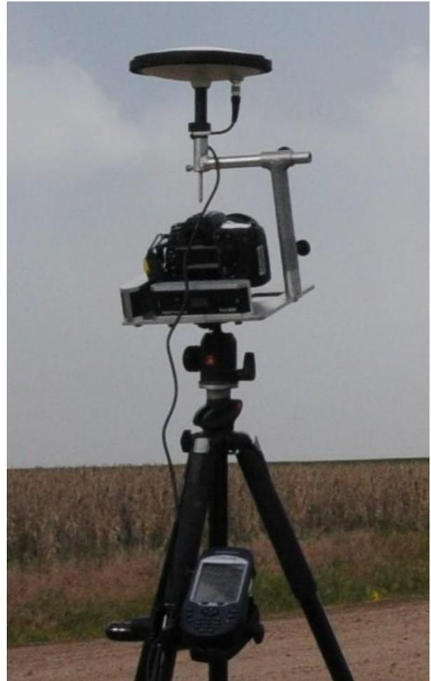
Figure 1. The photogrammetry camera base station including: 1) Promark3 GPS (bottom), GPS antenna (top), Nikon D300 camera fixed to a custom-built tripod mount with digital protractors on the rear and left side of the mount to measure pitch and roll.
