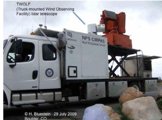
Figure 4. TWOLF mounted on the MWR-05XP radar truck, next to the phased-array antenna (orange). © H. Bluestein
