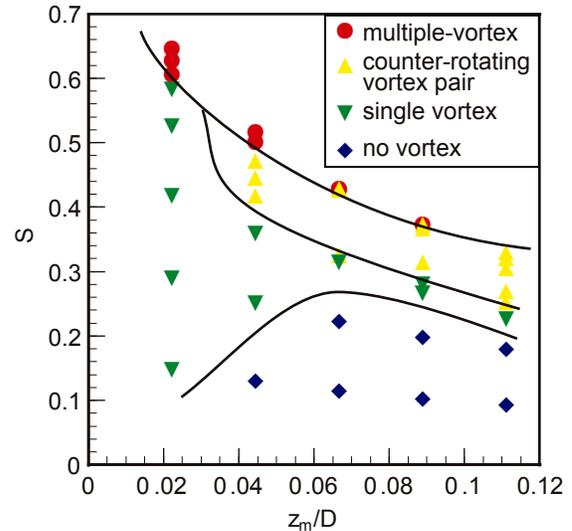
Figure 3: Regime of flow patterns realized in the mesocyclone simulator.
