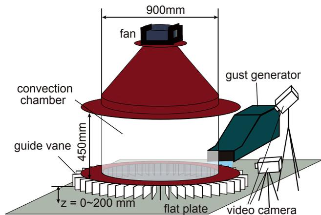
Figure 1: Mesocyclone simulator and gust generator.
