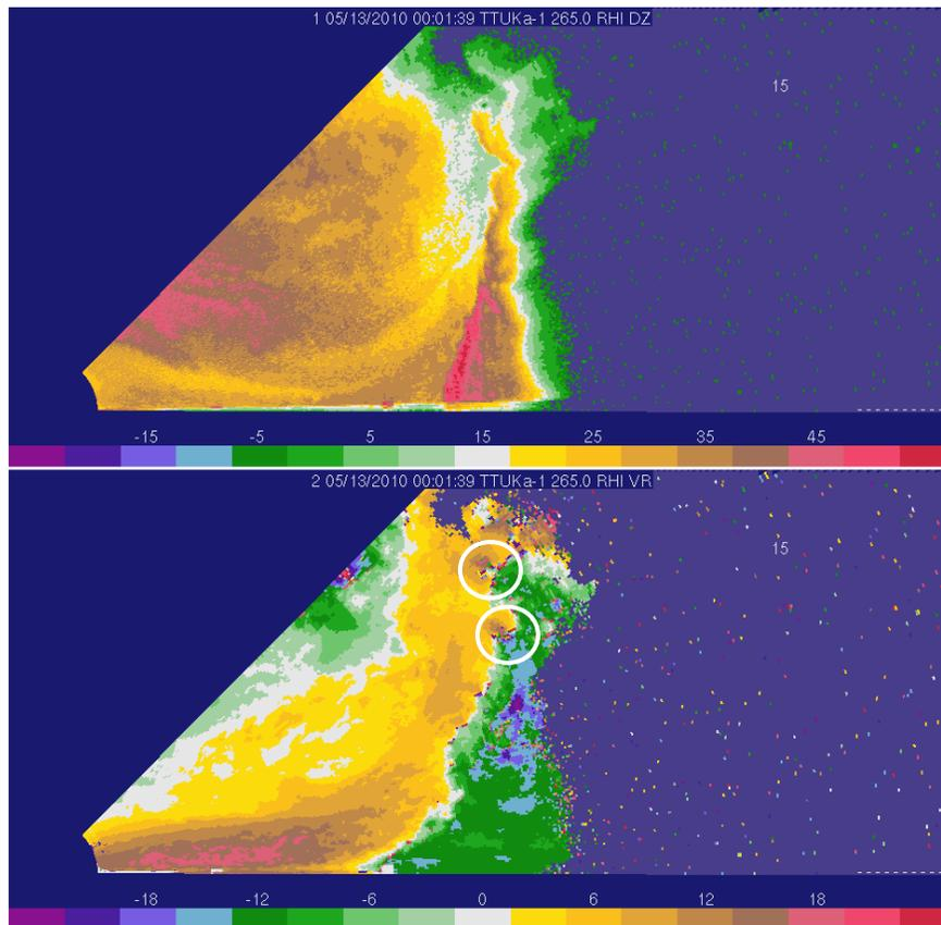
Figure 5 – TTUKa-1 RHI reflectivity (top, dBZ) and radial velocity (bottom, m s<sup>-1</sup>) of vertical vorticity maxima above the rear flank gust front of the 12 May 2010 near Willow, OK. The data were obtained at 0001 UTC (13 May 2010). Areas of strong horizontal vorticity are shown with white circles (discussed in text), and are ascending with time.
