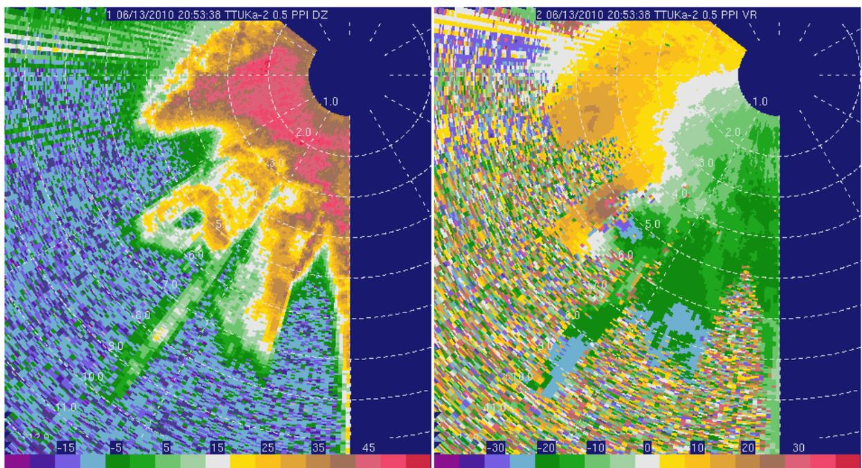
Figure 4 – TTUKa-2 reflectivity (left, dBZ) and radial velocity (right, m s<sup>-1</sup>) of a weak tornado north of Booker, TX on 13 June 2010 at 2053 UTC.
