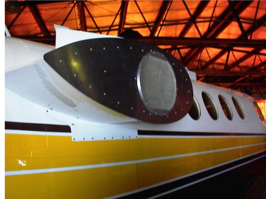
**Figure 3. The venetian blind polarization grid reflector lens mounted in the side window of the antenna pod of the University of Wyoming King Air aircraft.**
