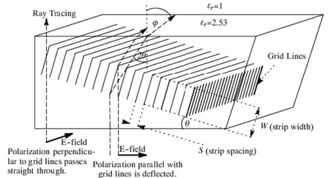
**Figure 1. Structure of the "venetian blind" polarization grid lens.**
