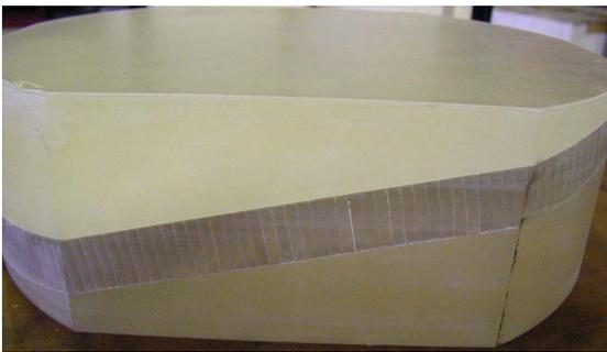
**Figure 2. The prototype venetian blind polarization grid reflector lens (side view)**
