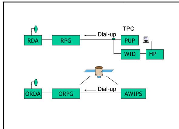
Figure 1. Schematic of existing radar data delivery system (top) with PC-based WID attached for file capture, and open system replacement (bottom).
