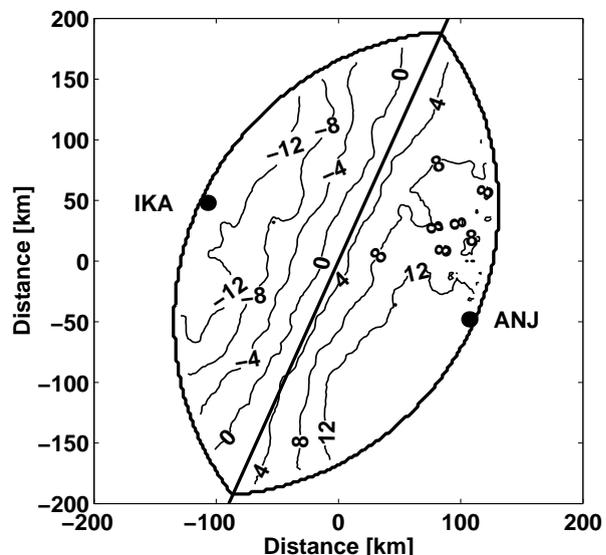
Figure 1: Difference of reflectivity between the Anjalankoski (ANJ,  $60^{\circ}54' N$ ,  $27^{\circ}6' E$ ) and Ikaalinen (IKA,  $61^{\circ}34' N$ ,  $23^{\circ}4' E$ ) radars. Contours of constant difference are given in steps of 4 dB. The radar locations are shown by black dots and the thick line connects points equally far from both radars.
