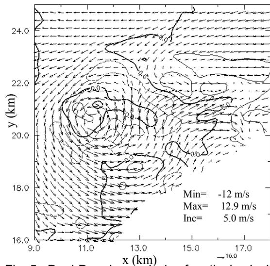
Fig. 5. Dual-Doppler analysis of vertical velocity and horizontal wind at 700 m for 20 May 1998, Bridgeport, NE tornado. Every third vector is shown. Domain as shown in Fig. 3.
