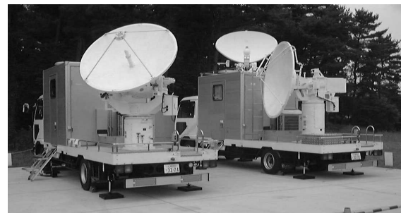
FIG. 1. Photograph of developed multiparameter radar system. X-band (right) and Ka/W-band (left) radar subsystems are mounted on 4-ton trucks. The antenna on the top of container of X-band radar is used for satellite communication.
