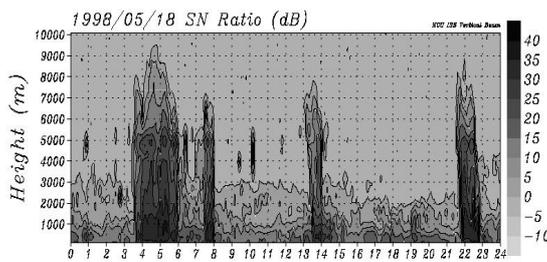
Fig 4. Time series of reflectivity of UHF radar on May 18, 1998
