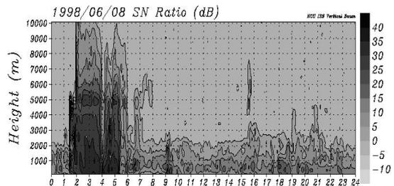
Fig 5. Time series of reflectivity of UHF radar on June 8, 1998
