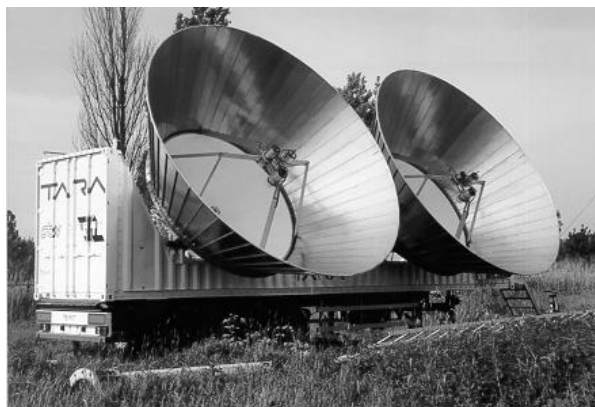
Figure 1: The TARA system. Clearly visible are the multiple feed systems to generate off-axis beams.
