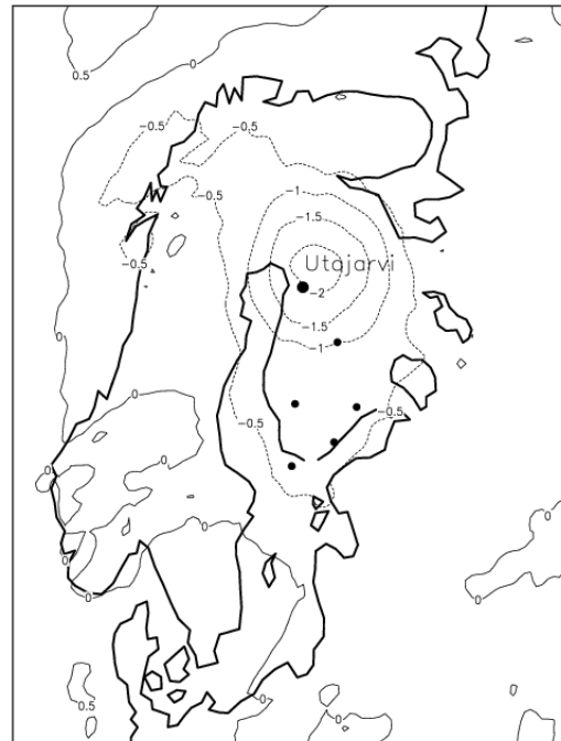
Fig. 1. Mean analysis increment of wind speed in October 1998 in m/s at about 860 hPa. The differences at the Utajärvi radar indicate systematic errors in the VVP winds.
