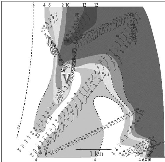
Figure 4. Subjective analysis of mobile mesonet dewpoint temperature as in Fig. 2 except for 2004-2020 UTC. Observations plotted every 6 sec. The vortex had a horizontal scale of approximately 2000 m. The X denotes location of 2005 sounding release point.
