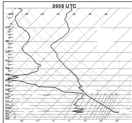
Figure 7. 2005 UTC M-CLASS sounding in skew  $T$ -log  $p$  format for 10 June 1999 released within the dryline mixing zone, approximately  $0.75 \text{ km}$  west of the large surface moisture differential. Winds as in Fig. 1.
