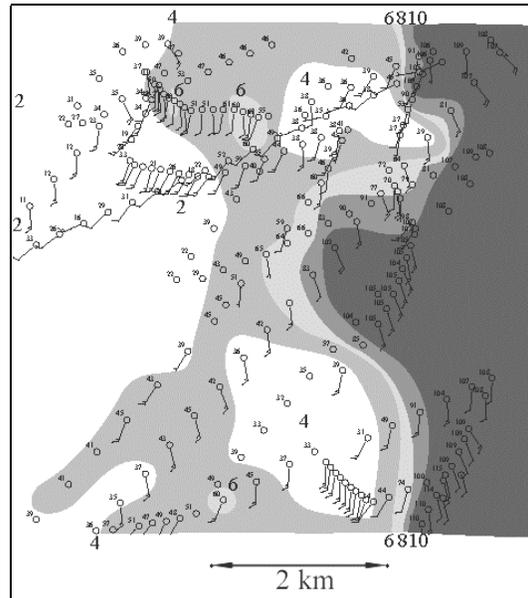
Figure 5. Subjective analysis of mobile mesonet dewpoint temperature as in Fig. 2 except for 2020-2033 UTC 10 June 1999. Note the tremendous moisture variability west of the largest moisture gradient.
