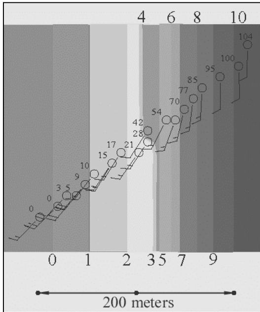
Figure 6. Mobile mesonet dewpoint temperature (tenths  $^\circ\text{C}$ ) and wind observations across the dryline at 2100 UTC 10 June 1999. No time-to-space conversion was used. Observations are 18-sec averages (3 observations) plotted every 6 sec. The mobile mesonet was traveling northeast at  $\sim 2.6 \text{ m s}^{-1}$ . Isodrosotherms shaded every  $1^\circ\text{C}$ . Winds as in Fig. 1.
