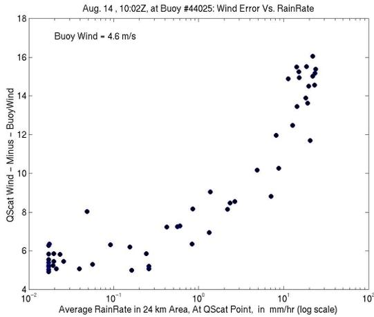
FIG 3. Rain-rate ( $\text{mmhr}^{-1}$ ) logarithmic scale as determined from WSR-88D at Upton, NY verses collocated scatterometer derived wind speed  $\text{ms}^{-1}$  at 1002 UTC on Aug. 14, 1999.
