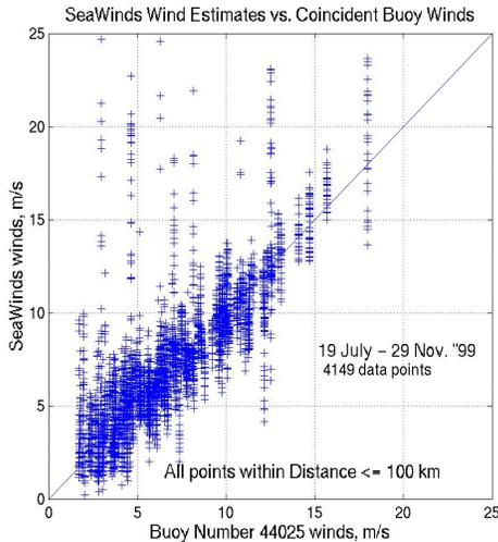
FIG 1. NDBC buoy 44025 wind speeds ( $\text{ms}^{-1}$ ) versus co-located scatterometer derived wind speeds for July 19 to Nov. 29, 1999.
