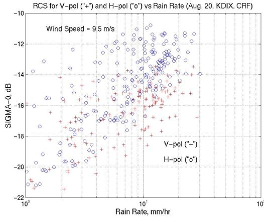
FIG 5. Scatterometer RCS reflectivity ( $\sigma^0$ ) (dB) versus NEXRAD derived rain-rate ( $\text{mmhr}^{-1}$ ) for Aug. 20, 2000. H-pol cells are designated "o" and V-pol "+". Coincident NDBC Buoy 44025 indicated  $9.5 \text{ ms}^{-1}$ .
