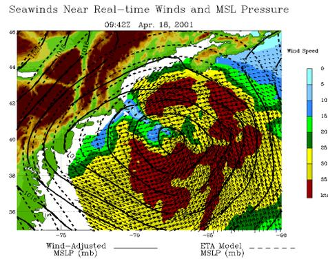
FIG 4. Example of scatterometer derived winds (kts) and MSLP (mb) from <http://www.coaps.fsu.edu/~zierden/qscat/> at 0942 (UTC) on Apr. 15, 2001. The wind speeds are color coded and binned to 5-knot increments to highlight standard winds speed levels used for advisories and warnings. The MSLP from the eta model is also overlaid.
