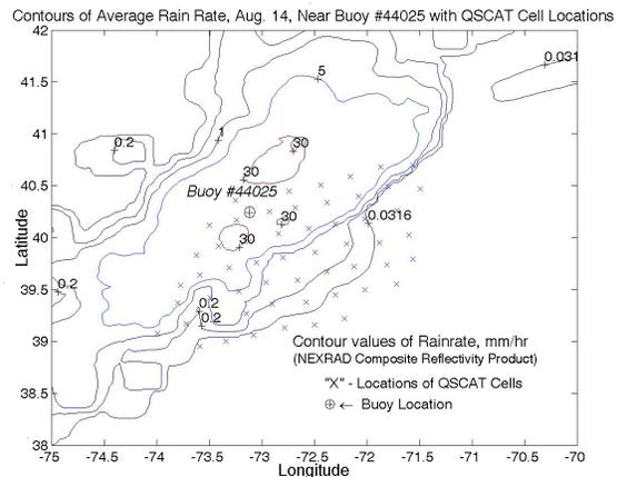
FIG 2. Rain-rate contoured to 0.03, 0.2, 1.0, 5.0, and  $30.0 \text{ mmhr}^{-1}$  overlaid with locations of center of scatterometer data cross-section points (x) and NDBC buoy 44025 (z) at 1002 UTC on Aug. 14, 1999.
