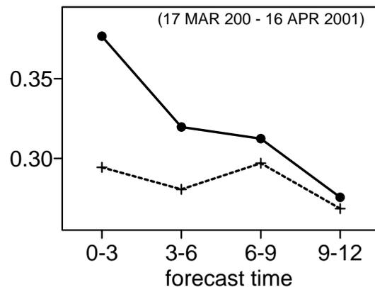
**Fig. 4 Threat scores of precipitation over 1mm/3hour from 17 Mar 2001 through 16 Apr 2001. Solid line is for the forecast from 4D-Var analysis and dashed line is for the routine forecast.**
