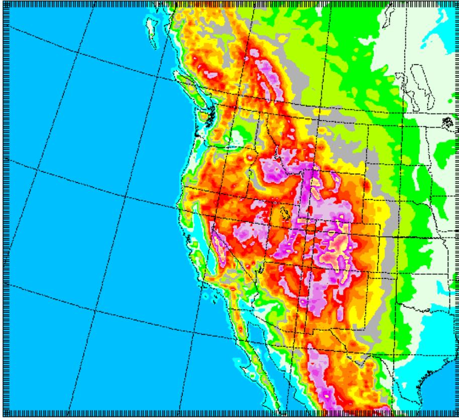
*Fig. 1. 20-km (217 x 197 gridpoints) PACJET RUC domain and topography (contour bands every 200 m).*
