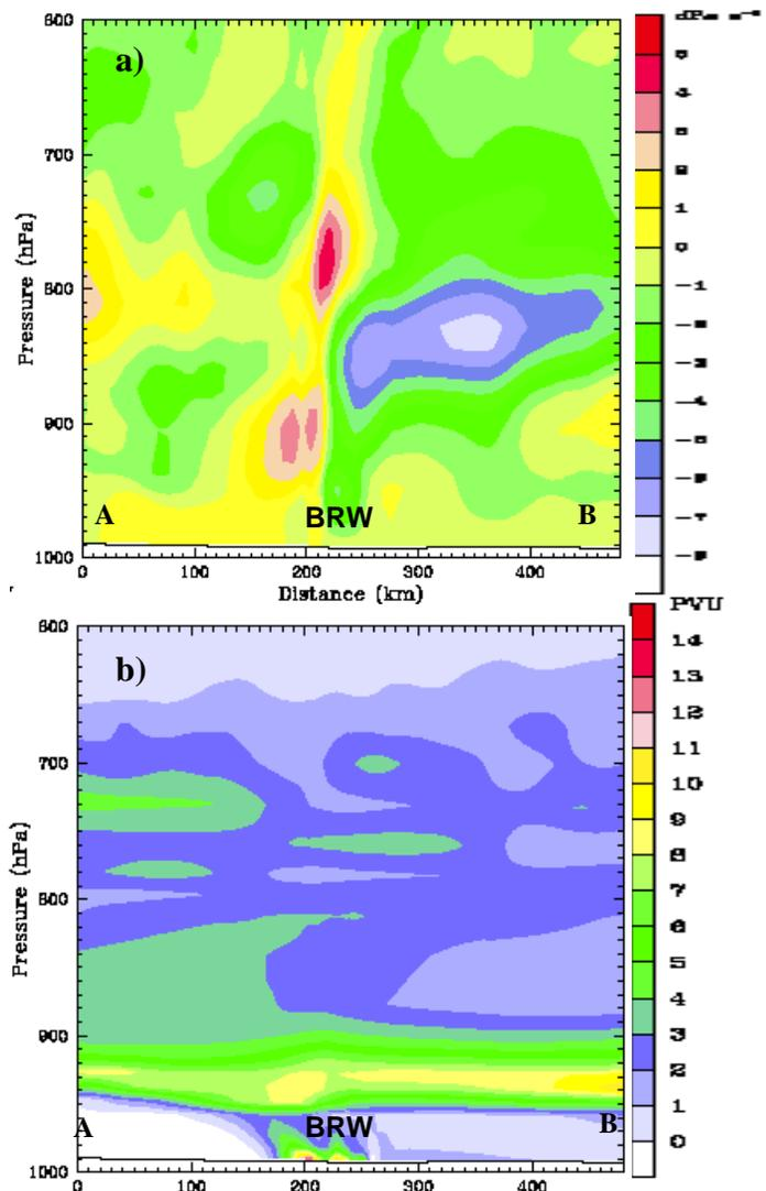
Figure 7. Cross sections through Barrow (marked 'BRW') of the a) vertical motion (dPa/s) and b) potential vorticity (PVU) fields at 12 UTC 1/8/01.
