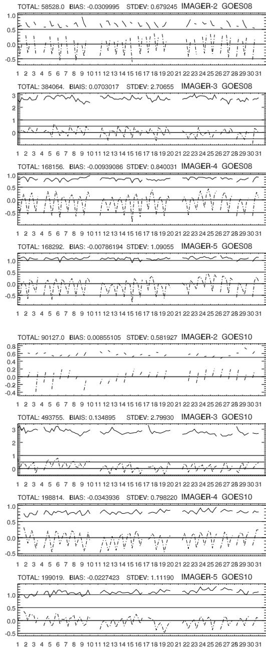
Fig. 1 Statistics of observed minus 6-h forecast calculated BT for imager channels of GOES-08 and 10 in March 2001 every six hours. Upper line is standard deviation; the mean is centered around zero. A bias correction was applied to the observations (see text). Only daytime data used for Imager 2. Number of cases, overall bias and standard deviation indicated. Data taken over oceans in clear areas for surface channels.
