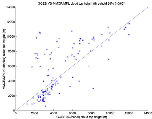
**Figure 2: A scatter plot comparing GOES and MPL/MMCR cloud top height with no data filtering. Little correlation is seen.**
