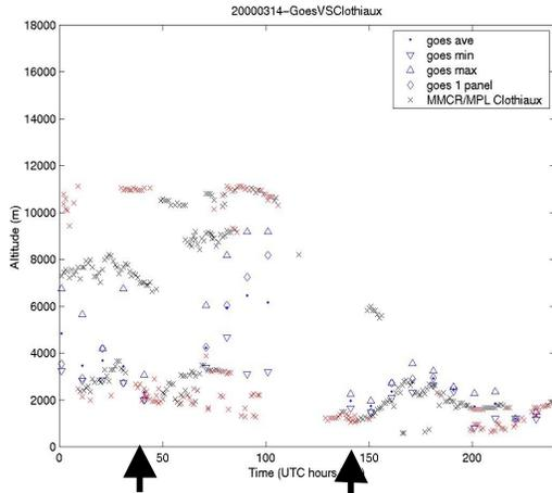
**Figure 5: Two instances of outliers that can be explained by examining the time series. Attenuation effects and multiple cloud layers led to the outliers.**
