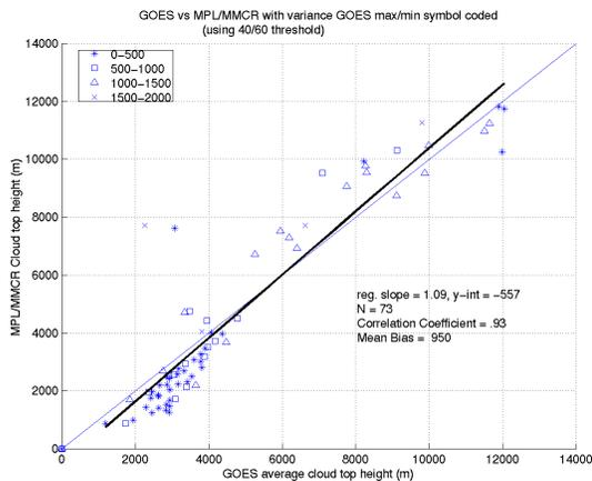
**Figure 6: A correlation coefficient of .93 and a mean bias of 950m is seen after application of filtering techniques and removal of outliers.**
