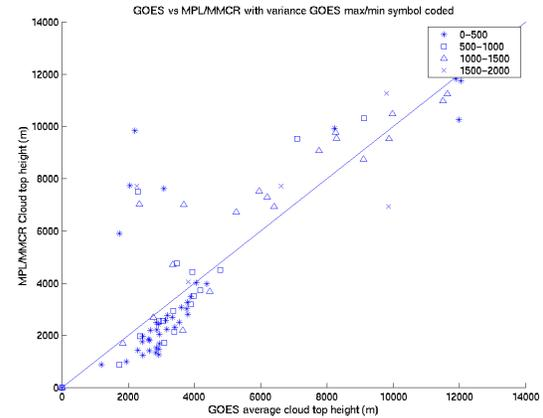
**Figure 4: Scatter plot using binning process for MPL/MMCR and filtering out multiple cloud layers. Amount of variance between sounder 3X3 FOV maximum and minimum cloud top height is symbol coded.**
