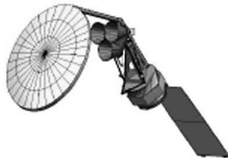
Fig. 6. Aquarius design concept showing the three feeds, the main reflector and the solar array.
