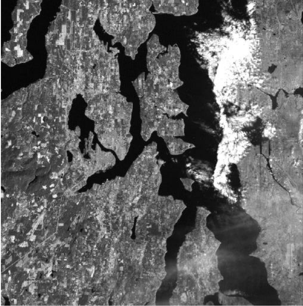
Figure 2. Landsat Band 5 ( \lambda = 1.65\mu\text{m} ) image collected 3/19/92 showing fog and low clouds around downtown of Seattle area.
