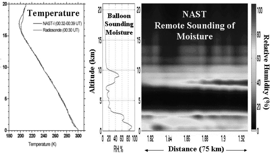
Figure 5: Retrieved and radiosonde Temperature profiles and a 75 km. vertical cross-section of atmospheric relative humidity near Andros Island Bahamas, on September 11, 1998.
