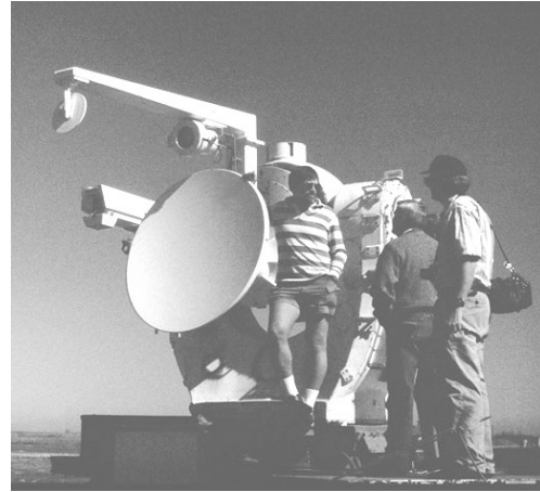
Figure 1. The NOAA/K radar's offset Cassegrain antenna. The rotatable phase retarding plate is located directly above the dish.
