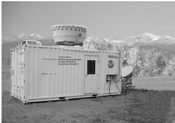
Figure 1. Photo of the MMCR Package showing the radar antenna (roof) and MWR reflector (right side).
