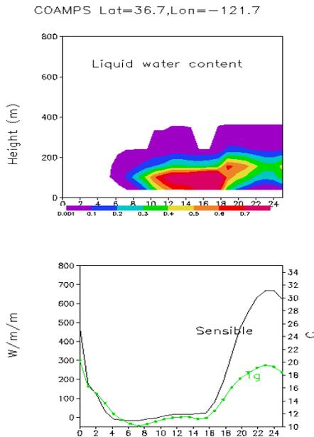
Fig. 6 Diurnal variation of clouds (above) and ground temperature ( $T_g$ ) and surface sensible heat flux, 6 July.
