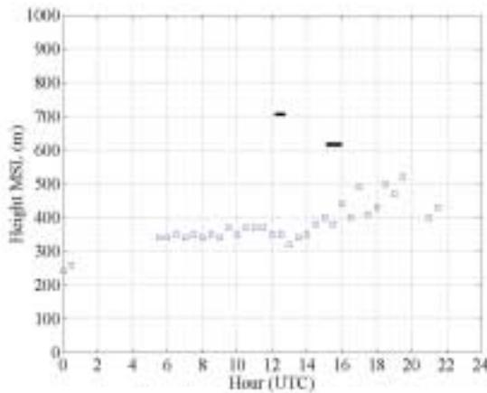
Fig. 1. Ceilometer measurement of cloud base heights (dot), and rawinsonde derived inversion base height (horizontal bars), 6 July, 1999.
