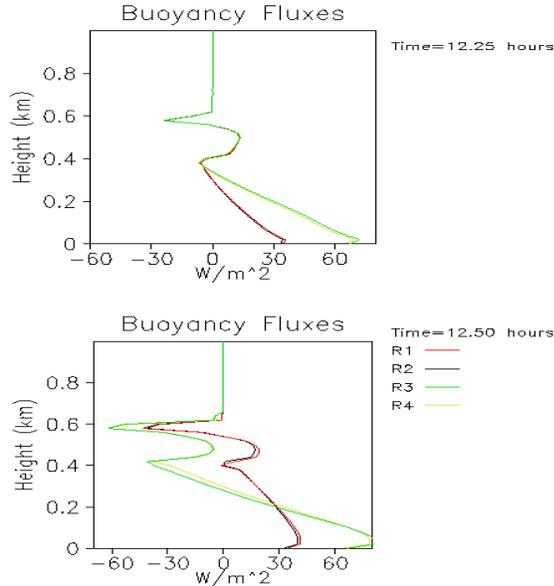
Fig. 3. Profiles of buoyancy fluxes at different times for different runs.
