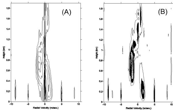
**Figure 2** An example contour plot of Doppler spectra vs. height before filtering (A) and after filtering (B). The large amplitude sea clutter signal in (A) has been removed leaving the clear-air spectra (B).
