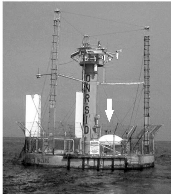
**Figure 1** Photograph of the 915-MHz wind profiler deployed on a 10-m discus buoy. The radar antenna sits beneath the radome indicated by an arrow.
