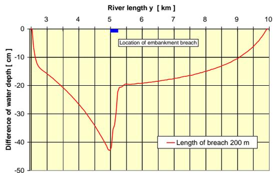
Figure 2: Reduction of water level by an embankment breach
