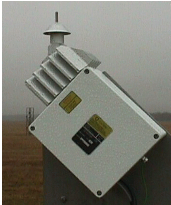
Figure 1. ASOS Icing Sensor
